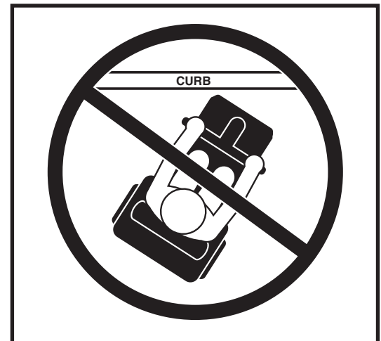
Figure 7. Incorrect Curb Approach
