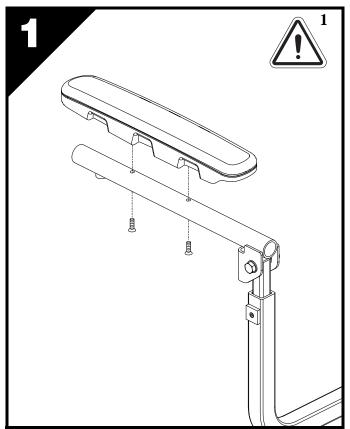
Remove the armrest cover and the accompanying securement screws from the armrest that DOES NOT contain the controller. Retain the armrest cover and discard the securement screws.
