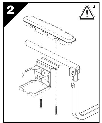
Install the Type D cup holder onto the armrest using the supplied securement screws and the retained armrest cover.
