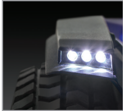
LED Fender Lights Standard with the Stretto, Edge 3, iLevel®, 4Front® and Edge Z
