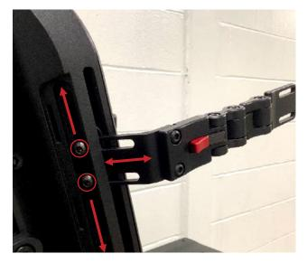
2. To adjust the <u>UniLink joints</u>, use a 4mm hex key to loosen the compression screws on the desired UniLink joints. Move to the desired position and tighten to lock in the position.
