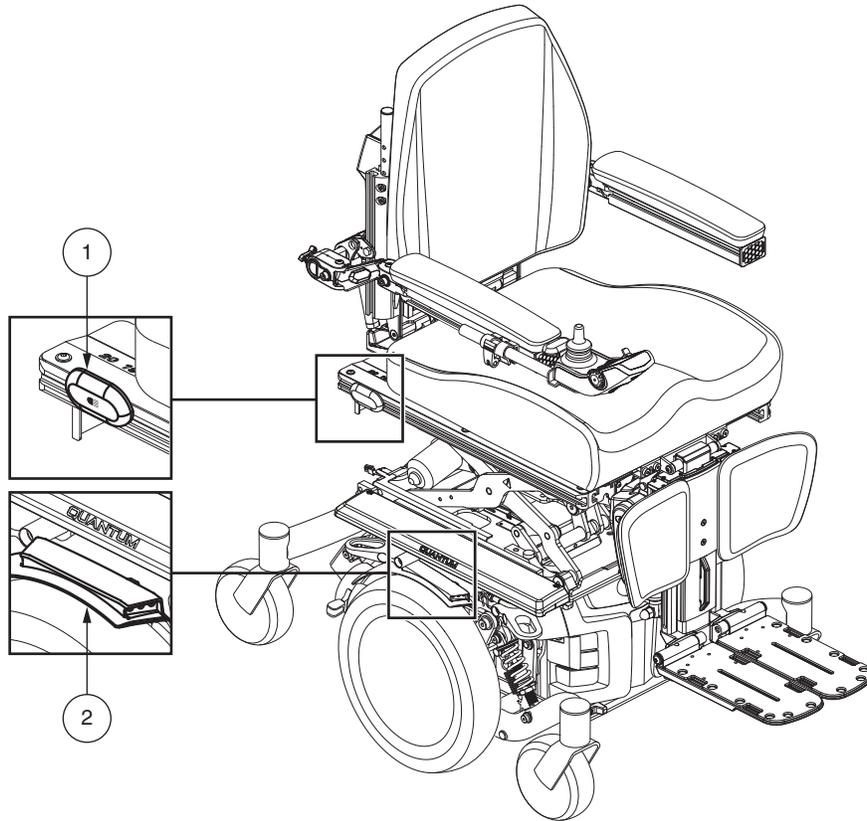
Figure 5. Q6 Edge 2.0 with Single Switch to operate Fender Lights.
