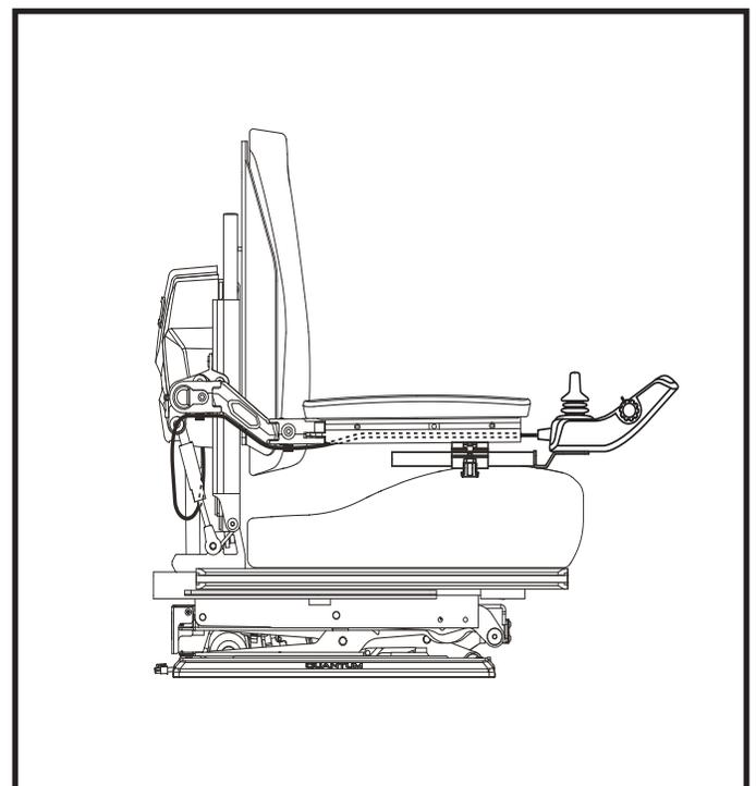
Figure 10. Controller Harness Routing on a Tru-Balance® Seat
