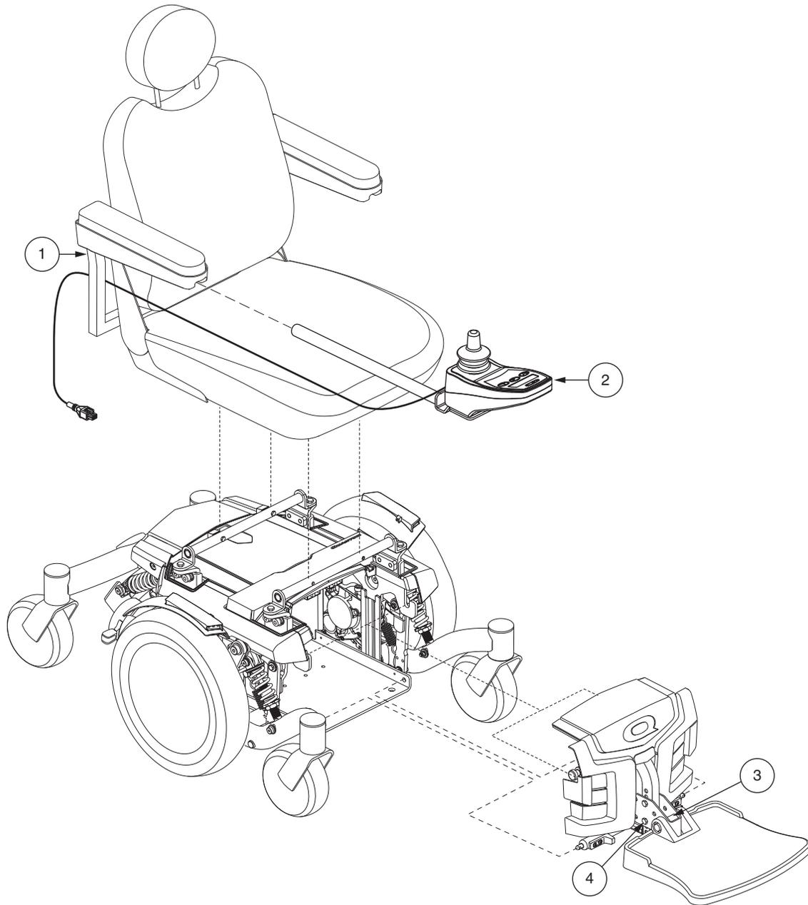
Figure 6. Q6 Series Assembly View
