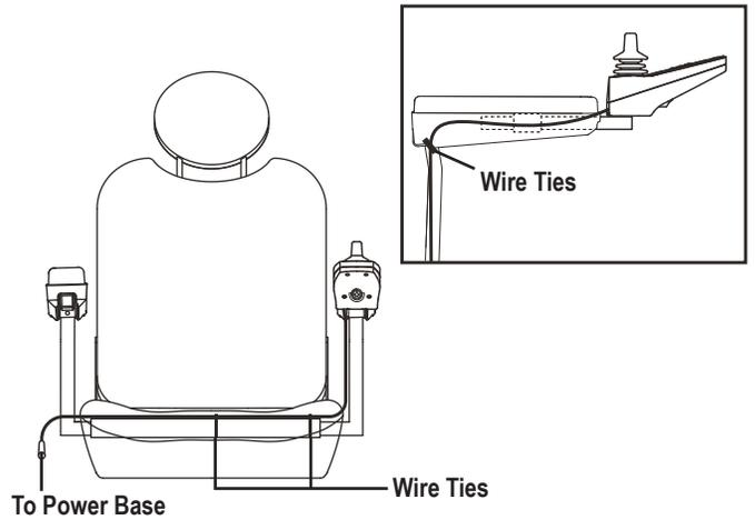
Figure 7. Controller Harness Routing on a Contour Seat
