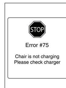
Figure 15. Q-Logic 3 Battery Charging Indicator
