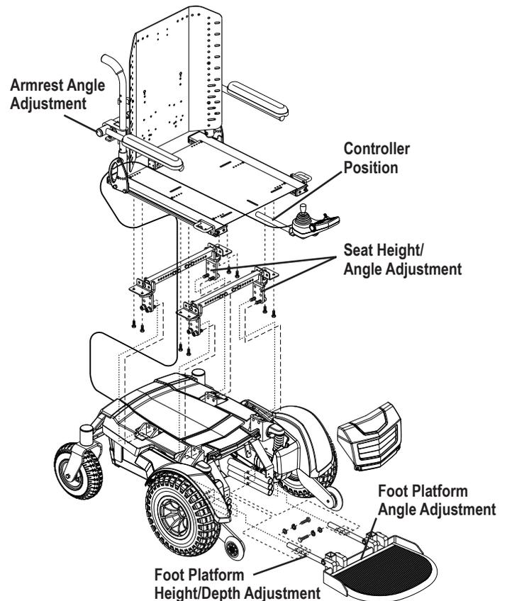
Figure 3. Assembly View (Synergy Seating System Shown)
