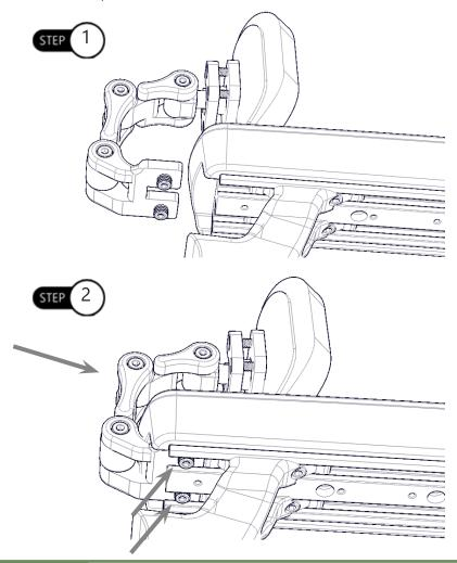
**NOTICE** Ensure that the heads of the M5x0.8x20mm SHS are facing out from the chair to allow adjustability while user is seated.
