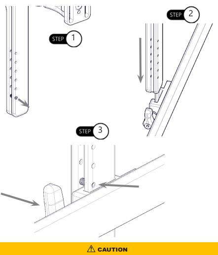
To avoid impact damage, ensure the ratchet handle is oriented parallel with the
